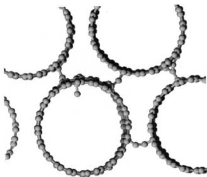
Fig. 6. Formation of molecular junctions in the bundle of single-layer carbon nanotubes in irradiating it with a beam of \text{Ar}^+ ions [114].
