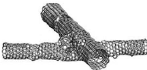
Fig. 5. Welding of single-layer carbon nanotubes by a beam of high-energy charged particles [19].
